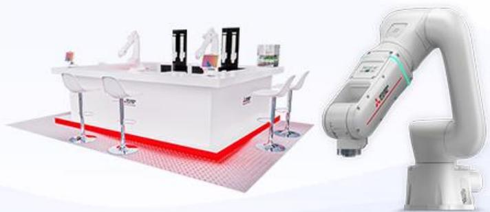
Collaborative Robots are designed to work directly with humans in a work environment simultaneously. This allows humans and Cobots to share tasks, work together in a production process, and increase work efficiency without endangering worker safety.
