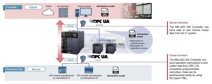
With the increased focus on cyber security for manufacturing systems, the MELSEC MX Controller is designed to meet IEC62443-4-2 standards\*4. It features secure OPC UA server support\*5, providing encrypted OT communication across platforms and ensuring protection from unauthorized access and data breaches. Security features include:
