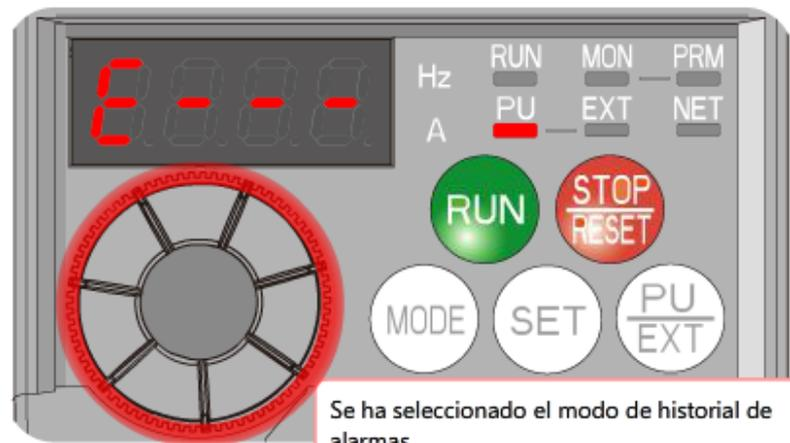
The diagram shows a control panel with a red digital display showing 'E- - -'. To the right of the display are indicators for Hz and A, and buttons for RUN, MON, PRM, PU, EXT, and NET. Below these are a green RUN button, a red STOP/RESET button, and three white buttons labeled MODE, SET, and PU/EXT. A red dial is highlighted with a red circle. Below the panel are three navigation arrows: a double left arrow, a single left arrow, and a single right arrow.
