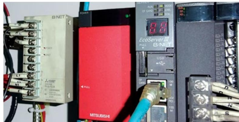
EcoWebServer III was introduced to visualize electricity consumption in the factories.
